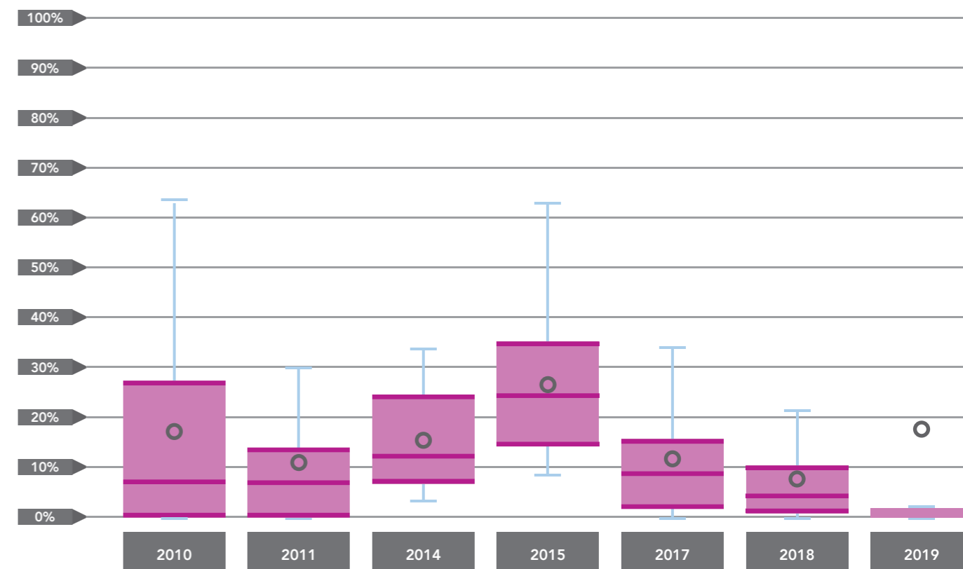
Figure 2: Share of total Br attributable to PBDEs. Data from 7 studies, 354 samples 4,6-8,10-12 . The boxes show the range from first to third quartiles, with the median dividing the box. Dots show the average values. Values below detection limit were considered as null.
